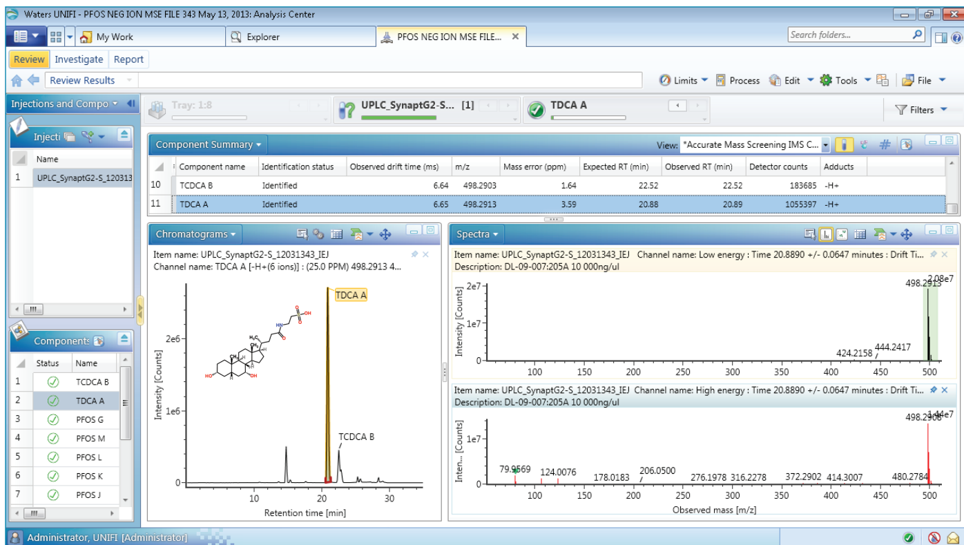
Figure 5. Ion mobility resolved characteristic fragmentation spectra of isobaric interference TDCA (A) at retention time 20.88 mins were generated using the combination of orthogonal ion mobility separation and UPLC chromatographic separation.
