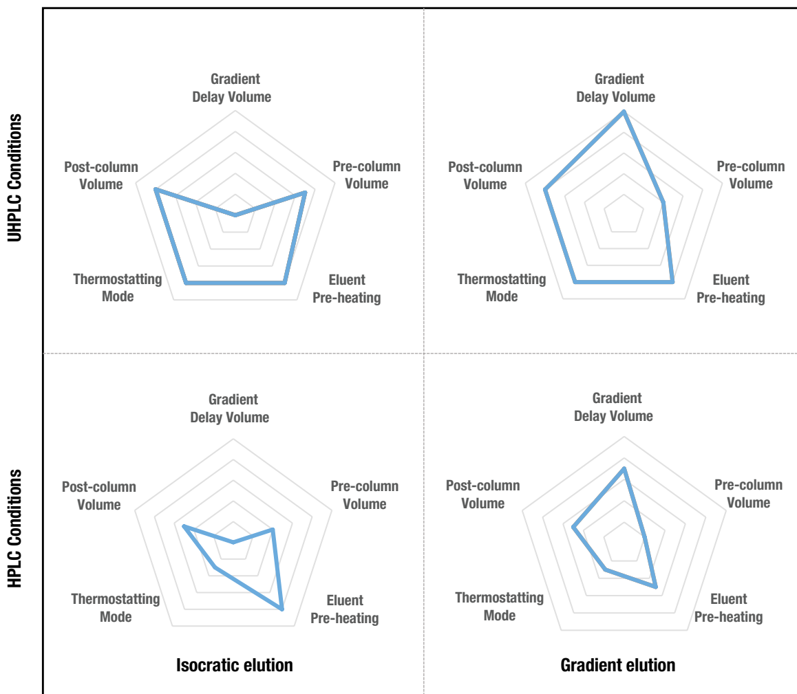
Figure 1. Instrument parameters and their importance for a successful method transfer. The further from the center of the graph, the more important the parameter. The importance value are estimates and dependent on additional method details such as separation temperature, flow rate, etc.
