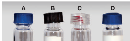
Examples of vial and closure misalignment/deformation. (A) SureStop vial self-aligning cap; (B) generic vial, cap tilt; (C) generic vial, septum dislodged; and (D) generic vial, deformed top.
