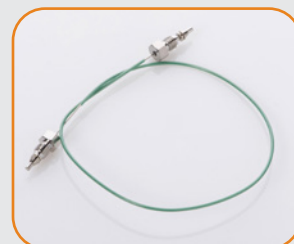
MODEL: 1290, 1260, 1200, 1100 CTS-21155 OEM 5067-4657 Capillary, 300mm x 0.17mm ID, w/Fittings (SST capillary pump to sampler)
