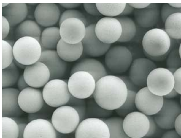
Figure 1 | FE-SEM image of Kromasil 100 Å, 3.5 μm particles.
