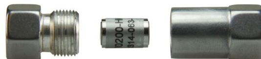
Figure 35. The 1.0mm i.d. and 2.0mm i.d. guard cartridges are for use with 1.0mm and 2.1mm i.d. analytical columns respectively, whereas the 4.0mm i.d. guard cartridges are for protection of 3.0mm and 4.6mm i.d. analytical columns. The hand-tightened holder allows for easy installation.
