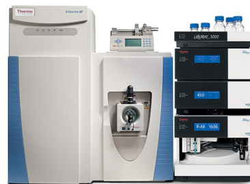
Thermo Scientific™ Q Exactive™ HF Hybrid Quadrupole-Orbitrap mass spectrometer and Thermo Scientific™ UltiMate™ 3000 RSLCnano system
